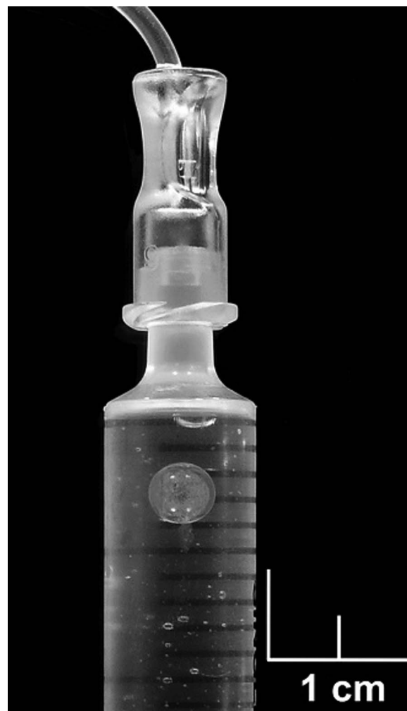
Figure 2 Bubbles present in an insulin pump cartridge and line following an increase in temperature from 4°C to 37°C. The insulin cartridge and line containing aspart insulin was cooled to 4°C in a fridge and then moved to an oven at 37°C.
