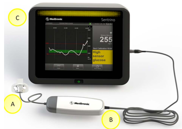
Figure 1 Components of the Sentrino continuous glucose management system: sensor (A), processor cable (B), and monitor (C).
